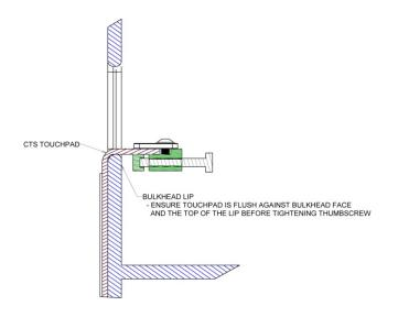
2.Place touchpad in pool. Ensure that touchpad is flush against the bulkhead face and the top of the bulkhead lip. Tighten thumbscrew to secure the touchpad in place.
