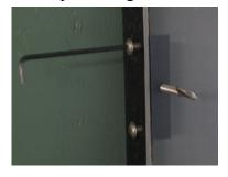
2. Attach brackets to touchpads using mounting holes in touchpad, as shown above (right). Tighten using the 7/32" hex key included with your order. Fully tighten bracket screws to secure bracket firmly in place. Use two brackets per pad for touchpads up to 77 inches (200cm) wide; use three brackets per pad for TP-78 and wider touchpads, or for higher level competition in which the athletes are likely to exert greater force in their turns. Touchpads can be stored with brackets attached.
