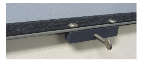
3. Place touchpad in pool. Ensure that touchpad is flush against the bulkhead face and the top of the bulkhead lip. Tighten thumbscrew to secure the touchpad in place.
