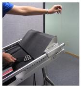
3. Adjust the fastener on the strap coming from the front of the RJP to allow the straps to connect underneath the block. Hook the loop of the strap from the front of the block onto the flat buckle, as shown. Repeat for the other flat buckle.
