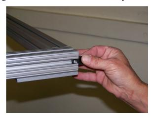
9) Add the end caps to the exposed ends (four on the base, and two on the top frame) by pushing the plastic screw through the end cap and firmly pushing that into the exposed end.
