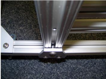
4) Slide the side panel on the base all the way to the corner bracket for the swivel wheel. Tighten the screws with the hex key.
