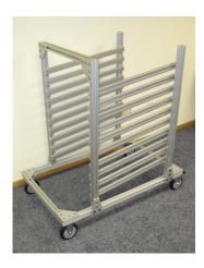
Orient the top rectangular frame so the corner brackets that are perpendicular to the frame are towards the end with the swivel wheels. Slide the T-nuts of those corner brackets into the top of the end posts, as shown above, left. Tighten the screws with the hex key.
