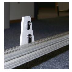
NOTE: The side panels have an X at the top of the end posts and the rails go smooth side to the inside.
