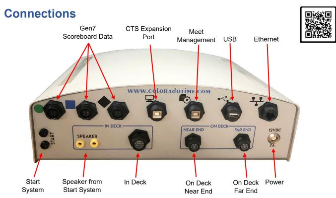
**Power Connection:** To connect the power supply to the Gen7 timer, line up the red dot on the power receptacle with the red dot on the connector on the power cord. Push in until it clicks in place. To disconnect the power cable, pull back on the sleeve on the connector (shown in red below) to unlock the connector from the receptacle then disconnect the power cord from the timer.
