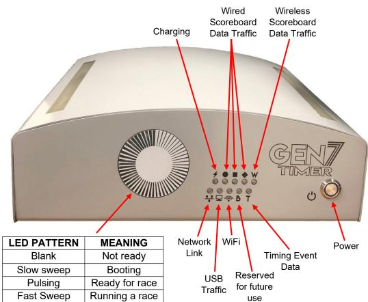
The LEDs on the front of the timer indicate data traffic and the state of the timer, as described above.
