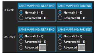
If using an On-Deck set up there are different mapping options available. Select **Advanced** and click the **Edit** button to open a dialog box where the lanes can be mapped so they are shifted as well as set to normal or reverse. For example, in an 8lane pool running 6 lanes, the lanes can be shifted so that lane 2 displays as lane 1, or if also set to reversed, lane 7 would display as lane 1.
