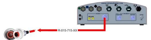
**For on-deck systems:** there are separate connectors for near end and far end serial cable harnesses. Serial cable harnesses may be chained together to support a primary and a backup harness for up to 20 lanes.
