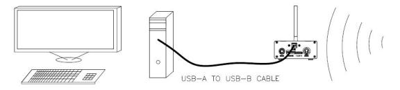
Connect the WA-3 to USB on the Display Link Plus (DL+) computer with a USB-A to USB-B cable (R-015-606). Power comes to the WA-3 via USB from the computer. Computer will assign a COM Port number that must be selected within Display Link Plus (DL+) as the input. (Refer to instructions in the back of this manual on locating assigned COM port.)
