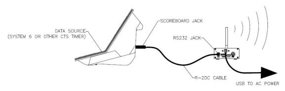
Connect the WA-3 to AC power with the USB power adapter, and to the System 6 with an R-DC cable.
