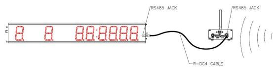
To display data on the LED-R scoreboard(s) or P01-style mini scoreboard(s), connect the WA-3 to a scoreboard with an R-DC4 cable. Power comes to the WA-3 from the scoreboard. If you have multiple scoreboards, connect them to each other with R-DC4 cables (ordered separately).
