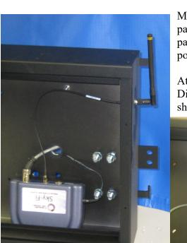
Many facilities place the WA-1 inside a scoreboard sign panel. To do this, enlarge the hole in the back of the sign panel enclosure to accommodate the data cable and the power cable.
