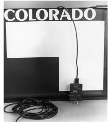
• When a fingertip is pressed against the surface of the touchpad, the entire red bar graph should illuminate; if it does not, you have an open touchpad (a touchpad that will not send a signal). Contact CTS customer support.
