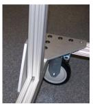
6. Using the level, make sure that the uprights are perpendicular to the ground, and tighten the screws with the 3/16" L-key.
