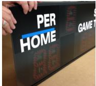
Note: When removing digits, do not grasp them by the LEDs; instead reach under the edge of the digit and pull up gently.
